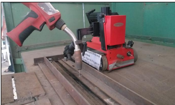
Fig – 2: Gas Metal Arc Welding Setup
