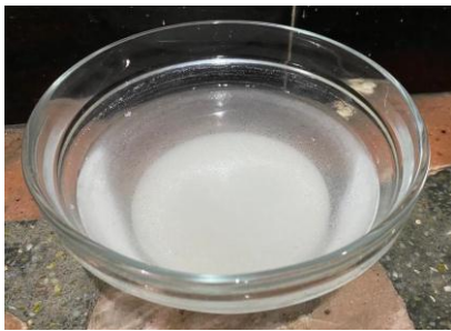
Fig-2: Bleaching powder diluted and supernatant liquid formed
