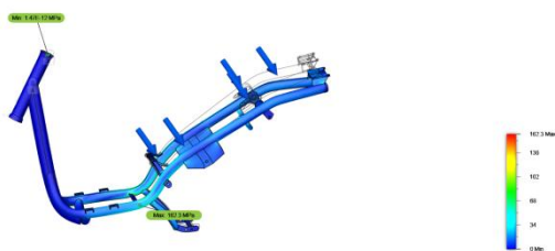
Fig 8: Stress analysis on chassis using fusion 360 software
