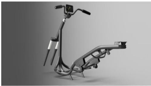
Fig 2: Iso metric view of scooter chassis
