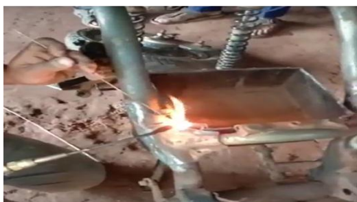
Fig 5: Fixing Battery Compartment
