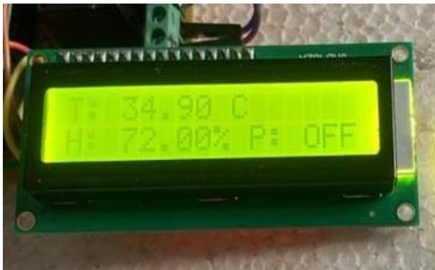
Fig 1 First Reading on hardware when mains power goes down
