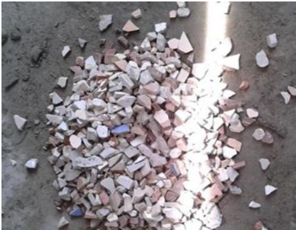
Figure 3.3: Ceramic Waste Tiles (CWT)
