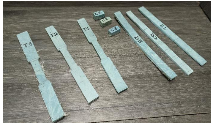
Fig-4: Test specimen prepared as per ASTM standards.
