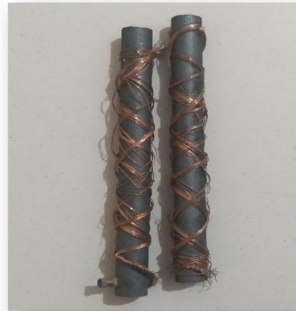
Fig -2: Graphite electrodes with copper wire as anode
