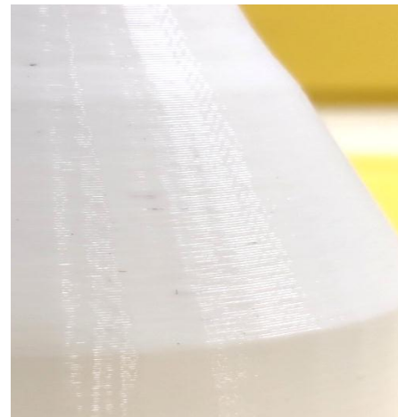
Fig -3: Image of the component showing staircase effect (Layer Thickness = 0.2 mm)
