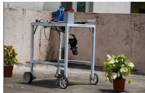
Rotation of the camera upto 180 degrees to obtain photos of the respective plant from all possible angles.
