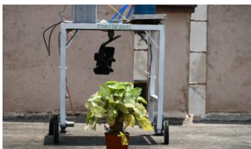
The prototype in motion and capturing the images of the plants using the rotoey motion with the help of Servo motor.
