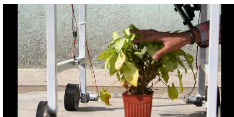
The ultrasonic sensors detecting the plant(obstacle)
