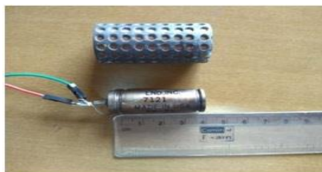
Fig. 2 A small sized GM Tube LND7121 with energy compensation shield [4]
