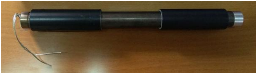
Fig. 3 A Longer GM Tube with higher sensitivity LND7807 with energy compensation shield [4]
