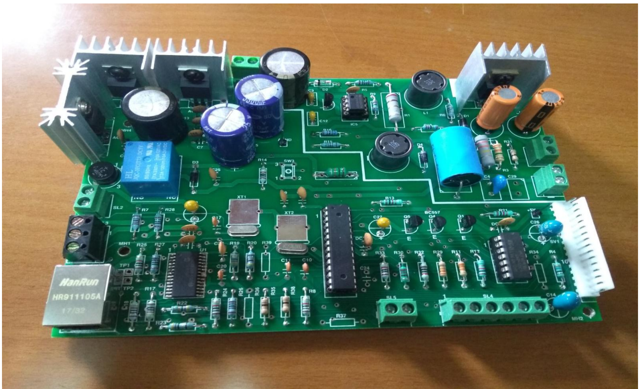
Fig. 11 Assembled Printed Circuit Board for the TCP/IP Ethernet and MODBUS Ethernet based model of Area Gamma Monitor
