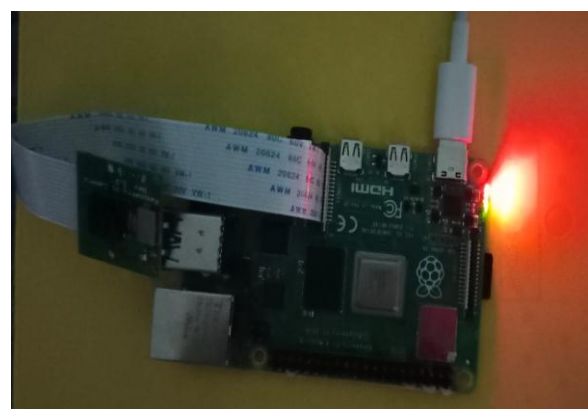
Fig no 2: Raspberry pi connected with Pi Camera
