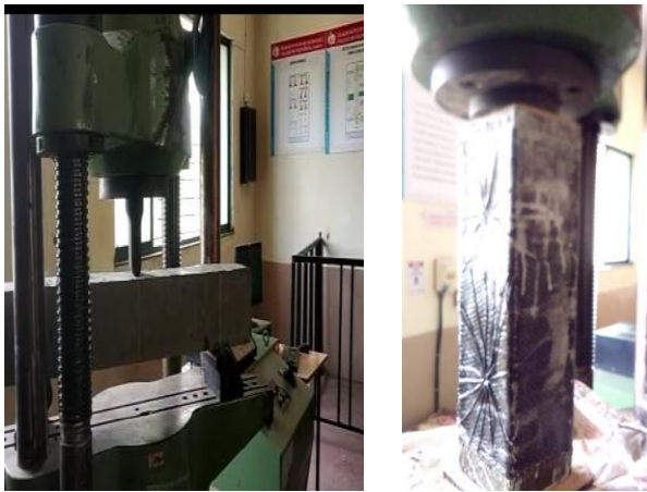
Fig.5: Testing of RC members
