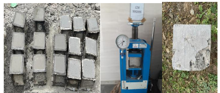
Fig -3: Cube casting testing and Failure pattern of cube
