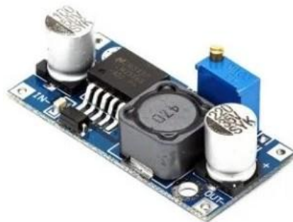
Fig 7: LM2596HVS Buck converter module
