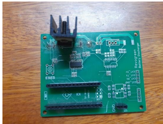
Fig 9: Discharger board PCB
