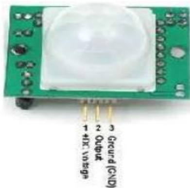
Fig-4 PIR motion sensor
