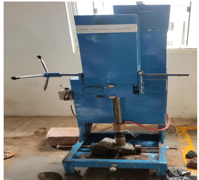
Figure 1: Core cutting machine
