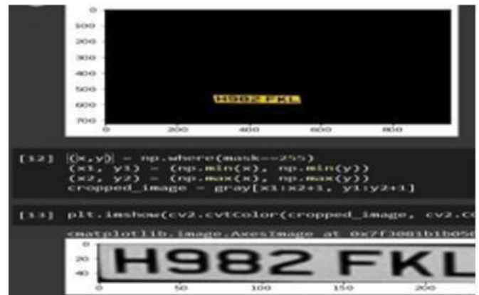
Fig-5.4.1 After applying the mask and cropping the number plate from the image.
