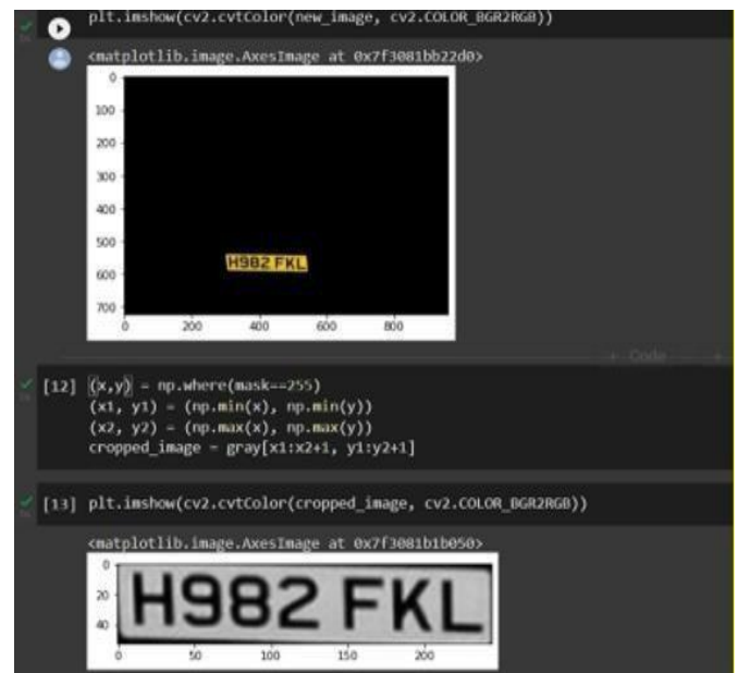
Fig-6.4 Applied the mask and cropped the number plate
