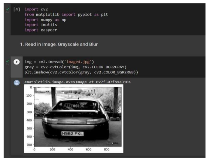
Fig-6.1 Read in image and then grayscale it using cvtColour and displayed it by using matplotlib.
