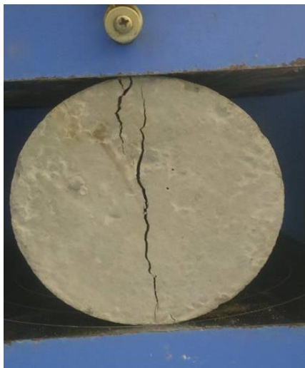
Fig: Split tensile strength test
