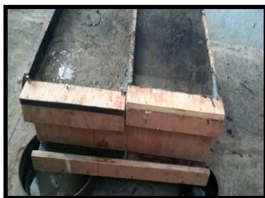
Fig 12 : Water percolation test on model
