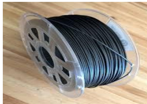
(b) PLA filament with Carbon Fibre Reinforcement
