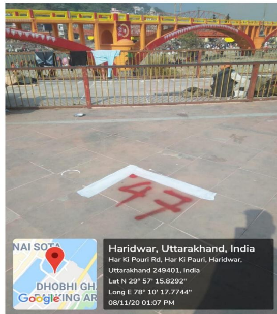
B. Ground Control Points(GCP) for getting absolute accuracy around 3-4 cm.
