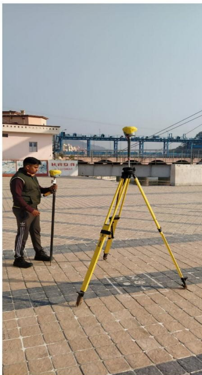
A. Temporary Bench Marks (TBM) for reference to the Ground Control Points (GCP) using DGPS.
