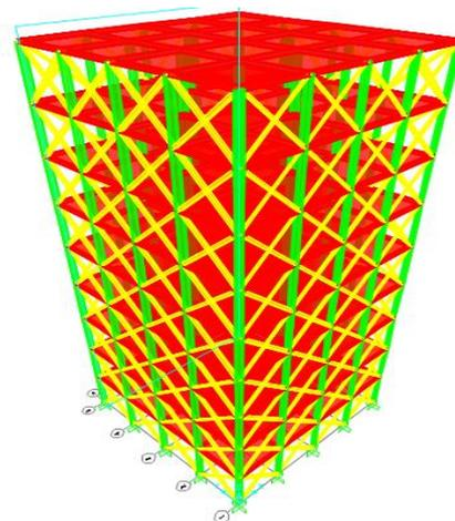
Fig -4: Bare frame with X-brace
