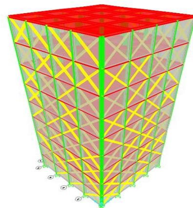
Fig -5: Bare frame with X-Brace and pre-cast infill
