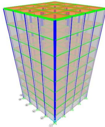
Fig -3: Bare frame with pre-cast pane infill
