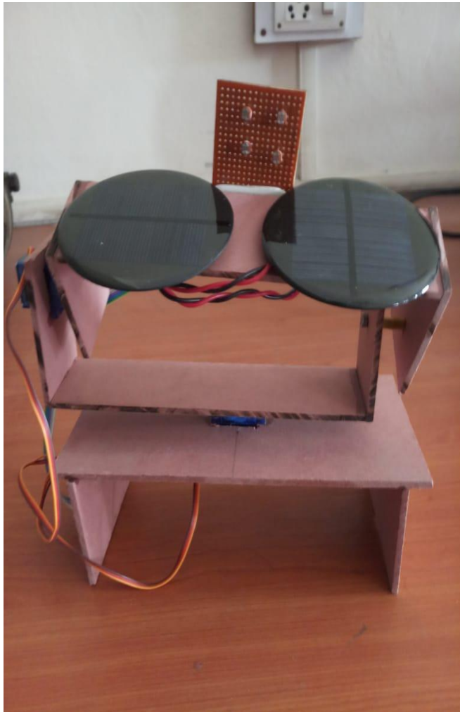
Fig. -2: Dual Axis Solar Tracking System
