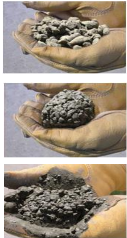
Figure 2. Samples of pervious concrete with different water contents: (a) too little water, (b) proper amount of water, and (c) too much water [3]
