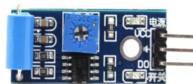
Fig-5: Vibration Sensor
