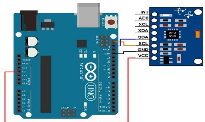
Fig -7: Interfacing MPU6050 Module with Arduino UNO6
