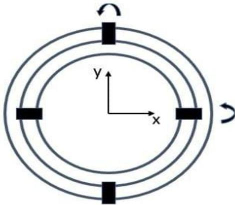
Fig -1: Conceptual design of gimbal ring
