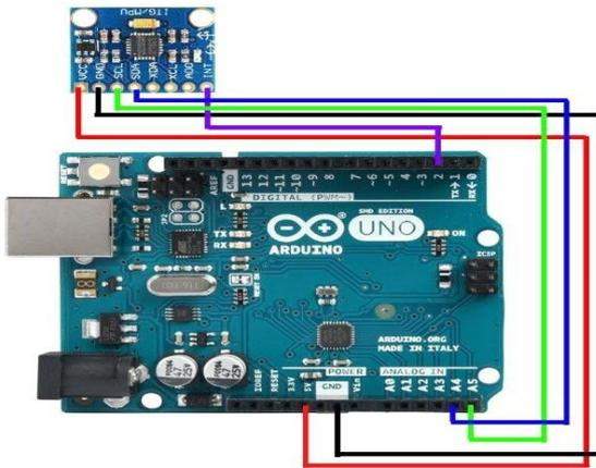
**Fig -8:** The circuit schematic diagram of the flight computer dubbed “Vector”
