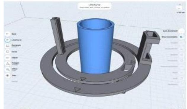
Fig -2: 3D design of Gimbal joints
