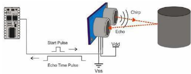
**Fig. 2 Ultrasonic Sensor Working**
