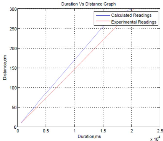
Fig. 7 Response of the Ultrasonic Sensor with Respect to the Obstacle Detection at Various Distances
