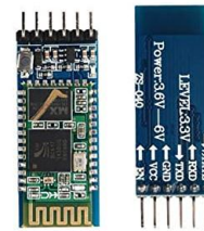
Fig -8: HC-05 Bluetooth Module
