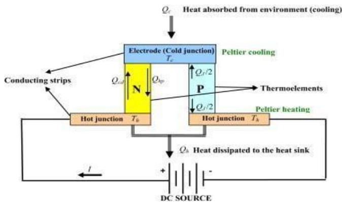
Fig. 5: Thermoelectric Cooling
