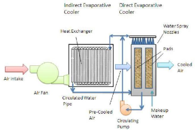
Fig 4: In-Direct evaporative cooling (Schematic structure)
