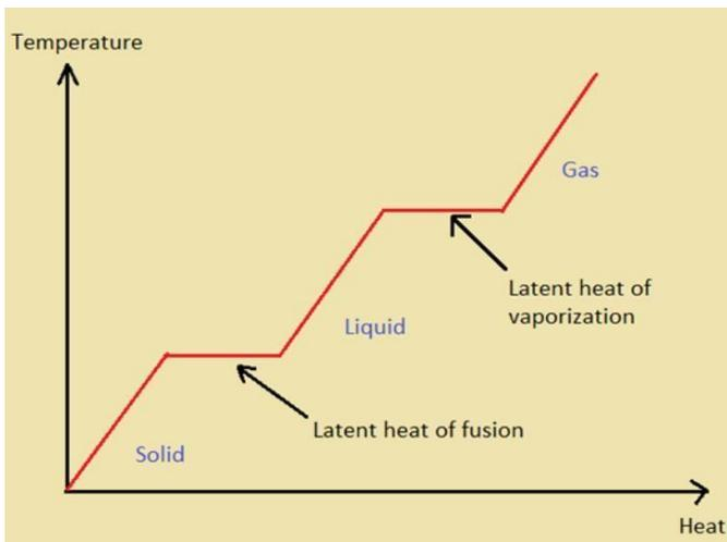
Fig 1: Latent heat of fusion
