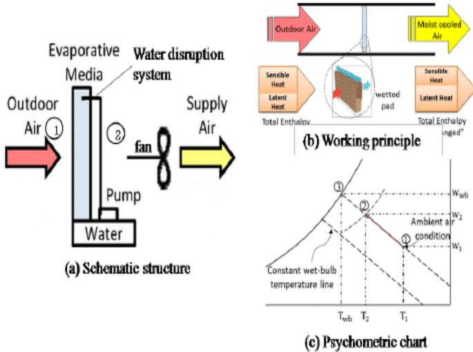
Fig 3: Direct evaporative cooling (a. Schematic structure, b. working principle c. psychrometric chart)
