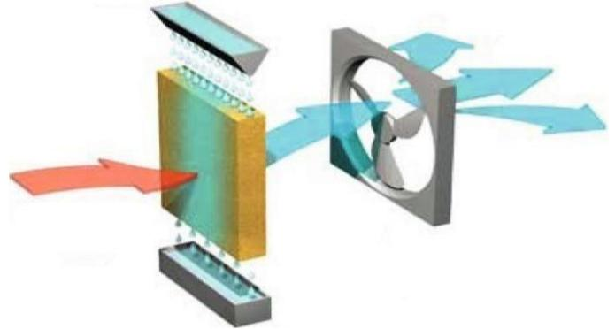
Fig 2: Direct evaporative cooling
