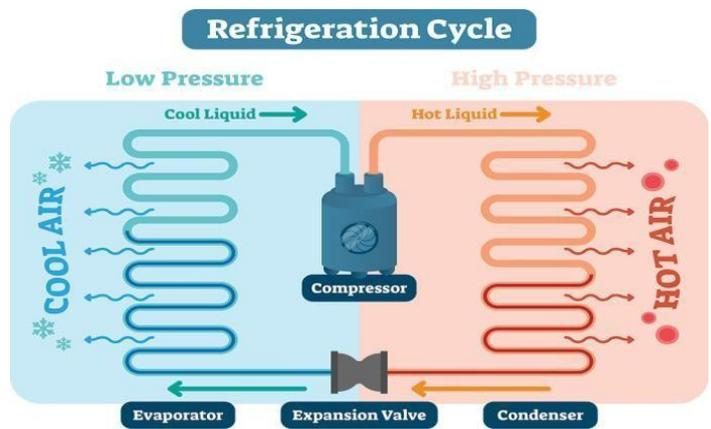
Fig 6: Refrigeration Cycle
