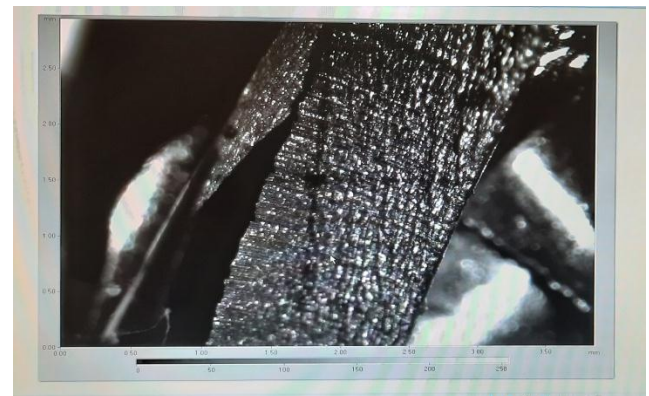
Fig -3: Chip surface preview with MahrSurf TS50 non-contact surface microscope
