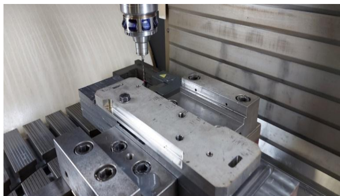
Fig -5: Measuring with IR touch probe on milling machine
