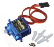
Micro Servo Motors are used to control the rotation of Camera module in 360-degree horizontal axis and 180 degrees in vertical axis
