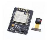
The ESP32 CAM Wi-Fi Module with OV2640 Camera is used for spying. It is a very competitive small size camera module that can operate independently as a minimum system and is widely used in various IoT applications.
