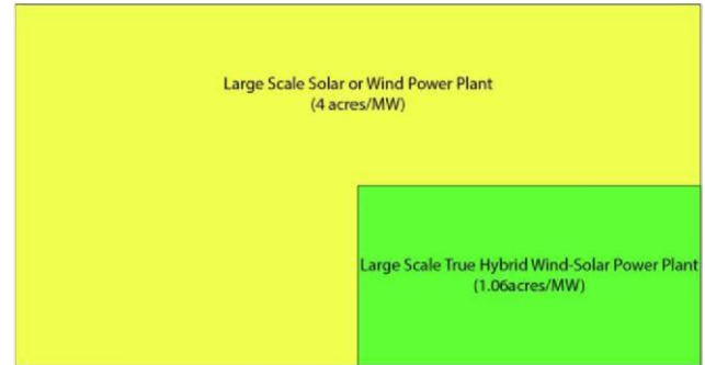
Fig. 10. THWS Generator Power Plant Land Size Comparison
