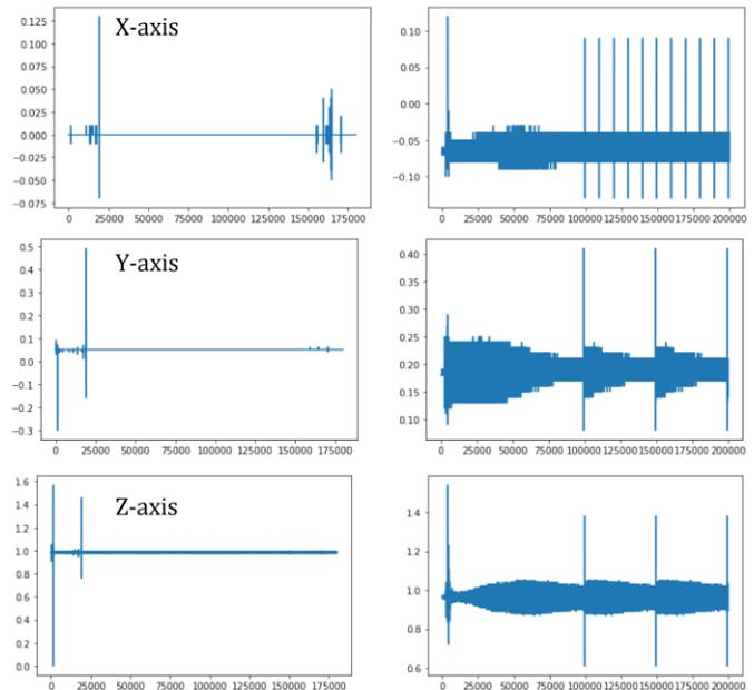
Chart -1: X, Y, Z -axis accelerometer reading with normal state and servo on.
