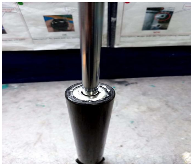
Fig - 2: Proper Sealing Operation
