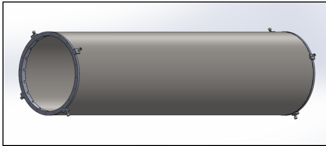
Fig- 5 : Ring Fixture Mounted on the Cylinder
