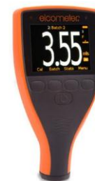
Fig-4: Elcometer 456 Coating Thickness Gauge Device
