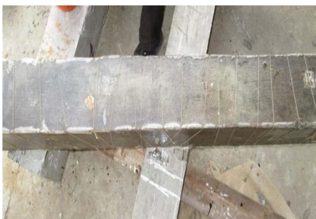
Fig -5: After applying Polyester Resin for bonding - 225 GSM
