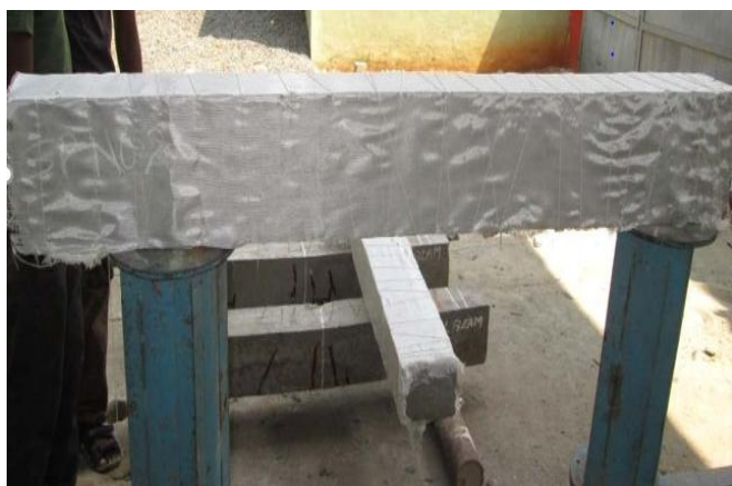
Fig -4: GFRP Wrapped Beam - 225GSM
