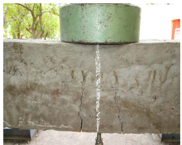
Fig-7: Crack Due to Ultimate Load
