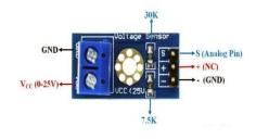
Needs no external components, Easy to use with Microcontrollers, Small, cheap and easily available.
