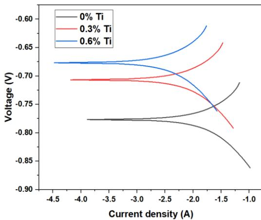
Figure 3 Corrosion curves of steel samples in H<sub>2</sub>SO<sub>4</sub>
