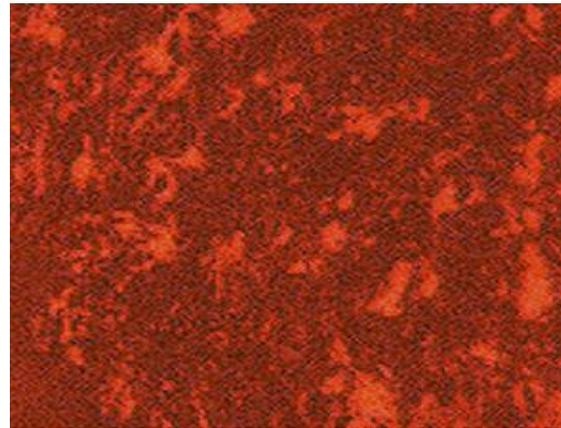
Figure 4 Micrograph of Ti<sub>0</sub> sample after corrosion
