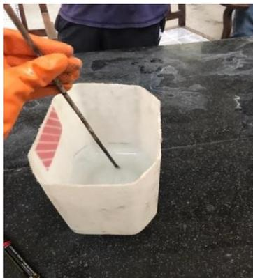
Figure 3.3 Making of alkaline solution and paste for normal consistency test
