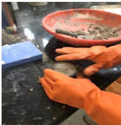
Figure 3.2 Making of alkaline solution and paste for normal consistency test
