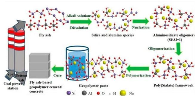
Figure 1.1 Chemical reactions between fly ash and Alkali solution
