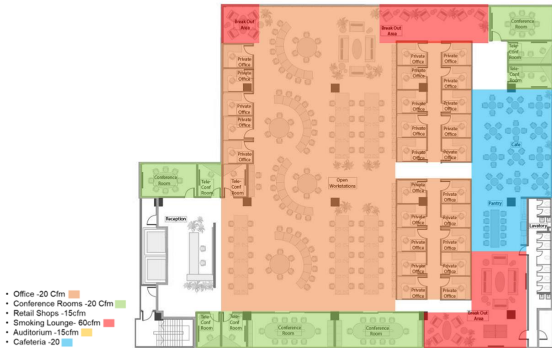
Fig. 3 ventilation rate/person in an office building as per green building codes (source- author)
