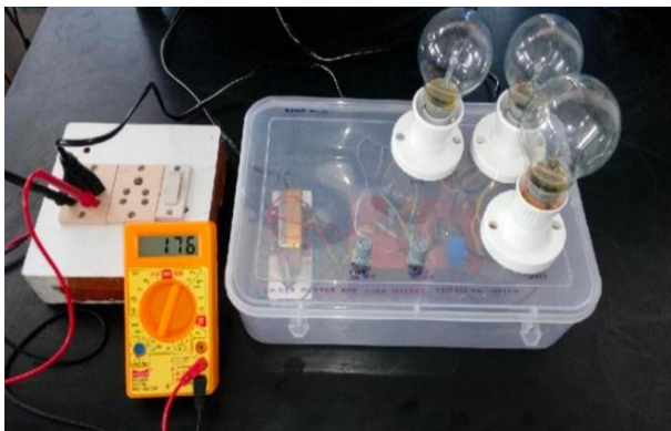
Fig.12. Proposed System when there is an over voltage in AC supply mains.
