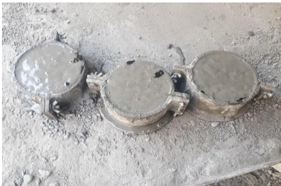
Fig -1: Casting of specimens
