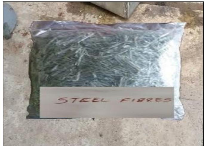
**Fig -2:** Steel fibers used in the project
