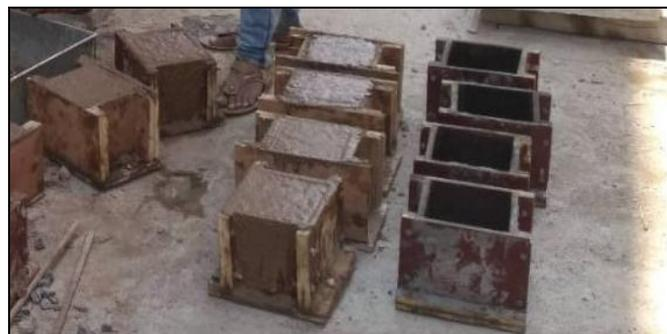
Fig -4: Mixing and casting
