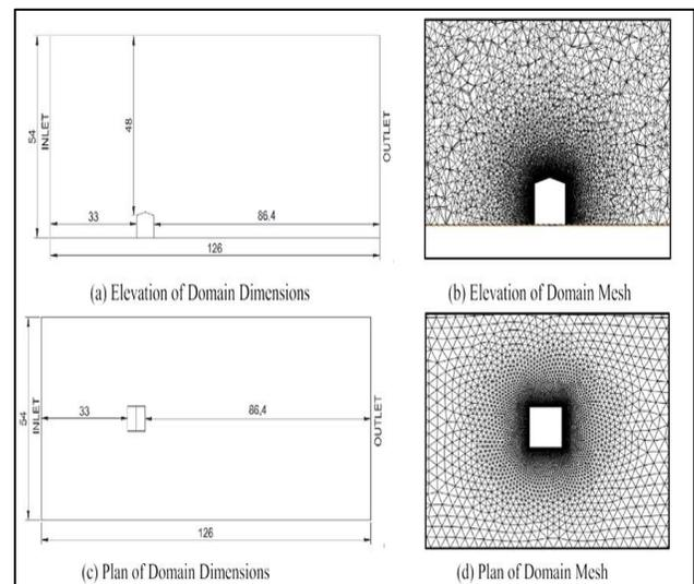
Fig. 1 Gable roof domain dimensions and mesh
