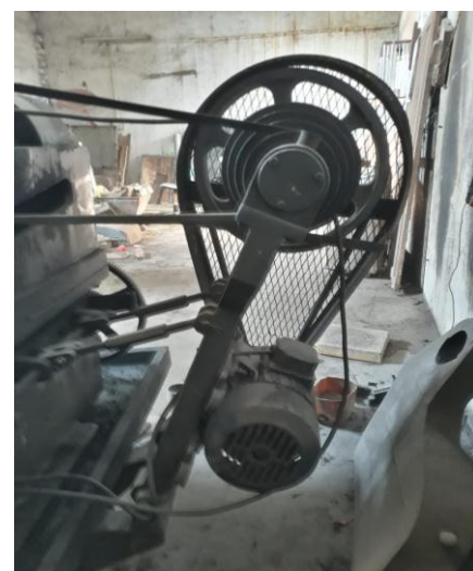
Fig -5: Motor And Drive behind Headstock
