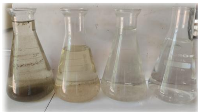
Fig -5: Influent (left) and effluent from the three units in series for greywater
