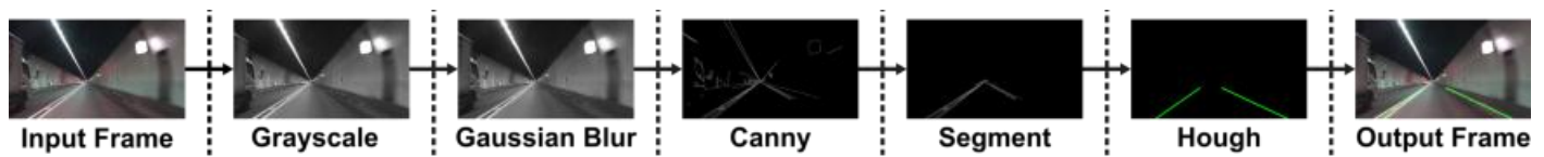
Fig.6 Lane Detection Pipeline
