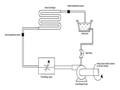
Fig 1: Simplified layout of testing aparatus
