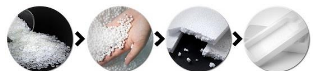
Fig-2 Producing Expanded Polystyrene Sheets and Molds
